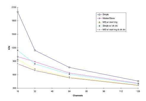
The chart above shows the sampling rates possible for different hardware setups using one DIO-128 board. The chart shows the rates to sample scans. Time to transfer the scans are shown below in Data Transfer Rates.
