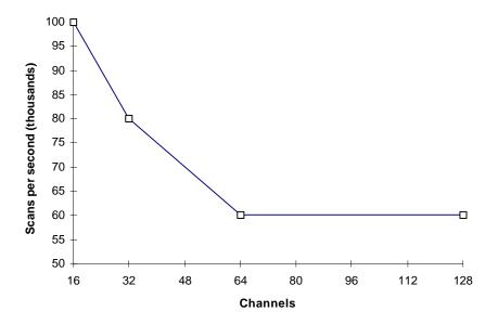
The chart above shows the number of scans per second that were transferred from the FIFO on the DIO-128 board to LabVIEW. These transfer rates were observed while running on a 166 MHz pentium machine with 32 Meg of RAM under Windows 95.
